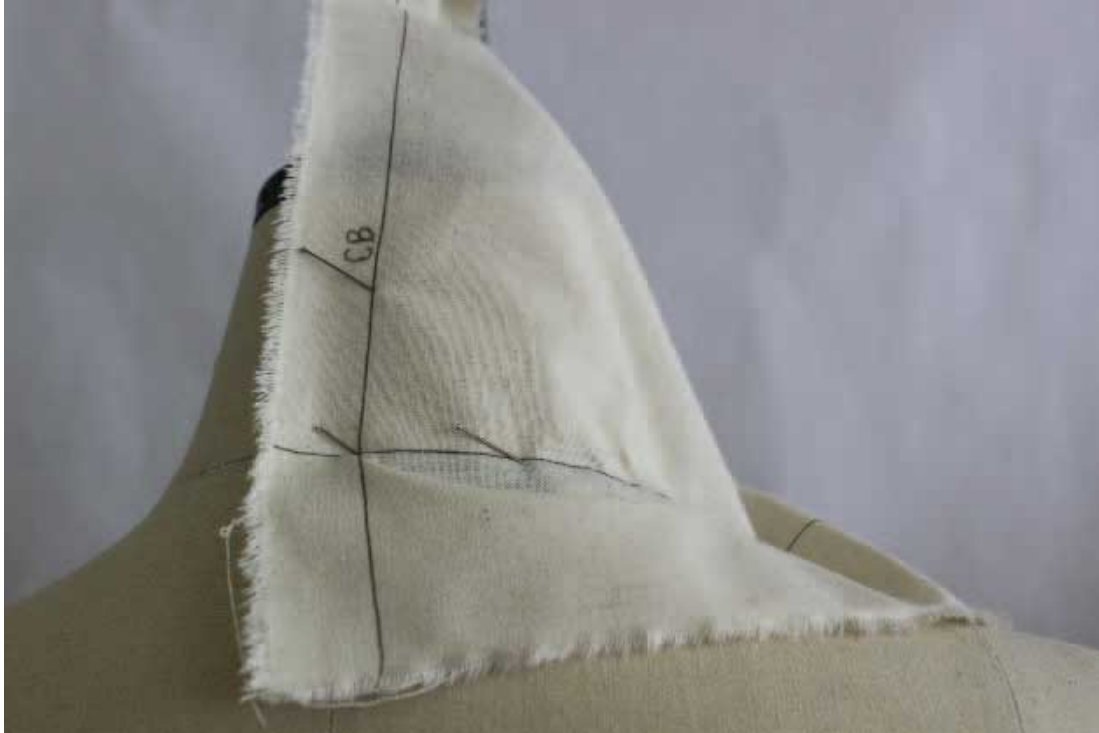
Fig. 10.19 Pinning roll line position and smoothing calico around back neck to neck point.
