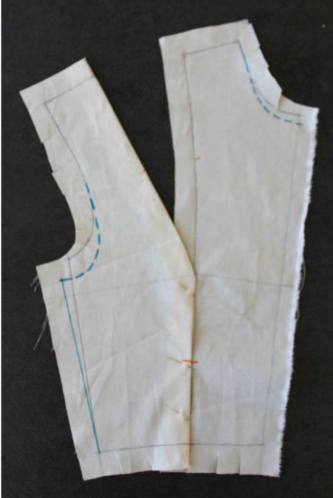
Fig. 6.6 Flat dart drape showing darts running from shoulder to BP and waist to BP.
