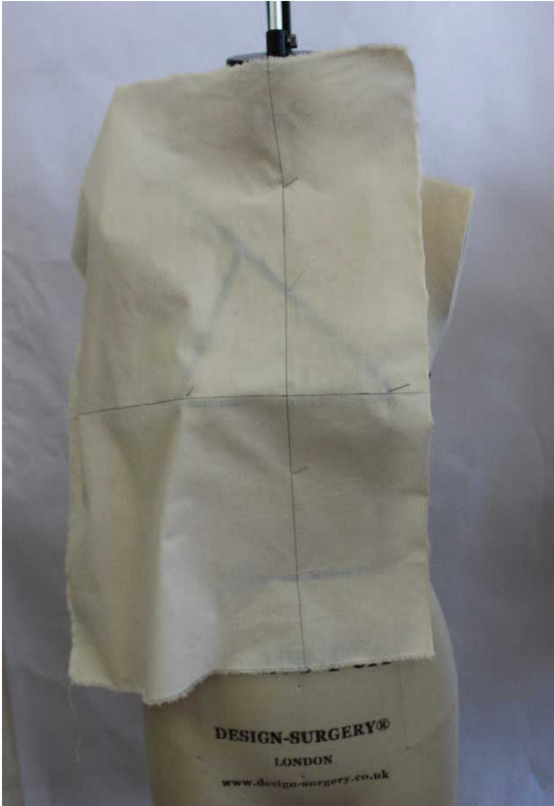
Fig. 6.48 Aligning calico to drape right front panel of asymmetric design with dart.
