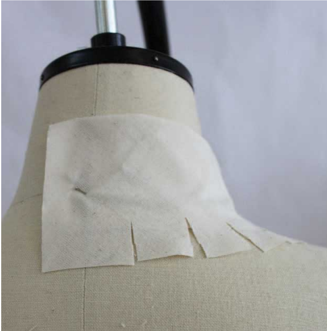
Fig. 10.14 Snipping into neckline to release tension and achieve fit for stand collar.
