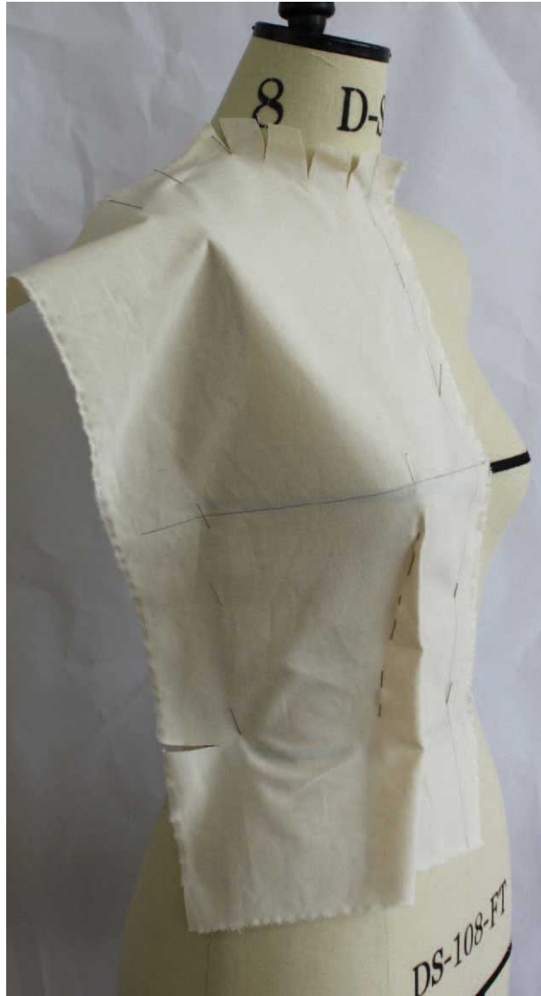
Fig. 6.17 Pinning waist dart in and snipping into waist from side allowance to release tension.
