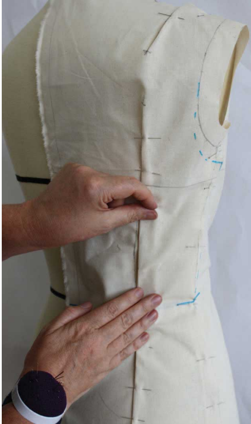
Fig. 5.10 Pinning seams and darts together on longline bodice; the pins go in and out through all the fabric layers and the stand cover.
