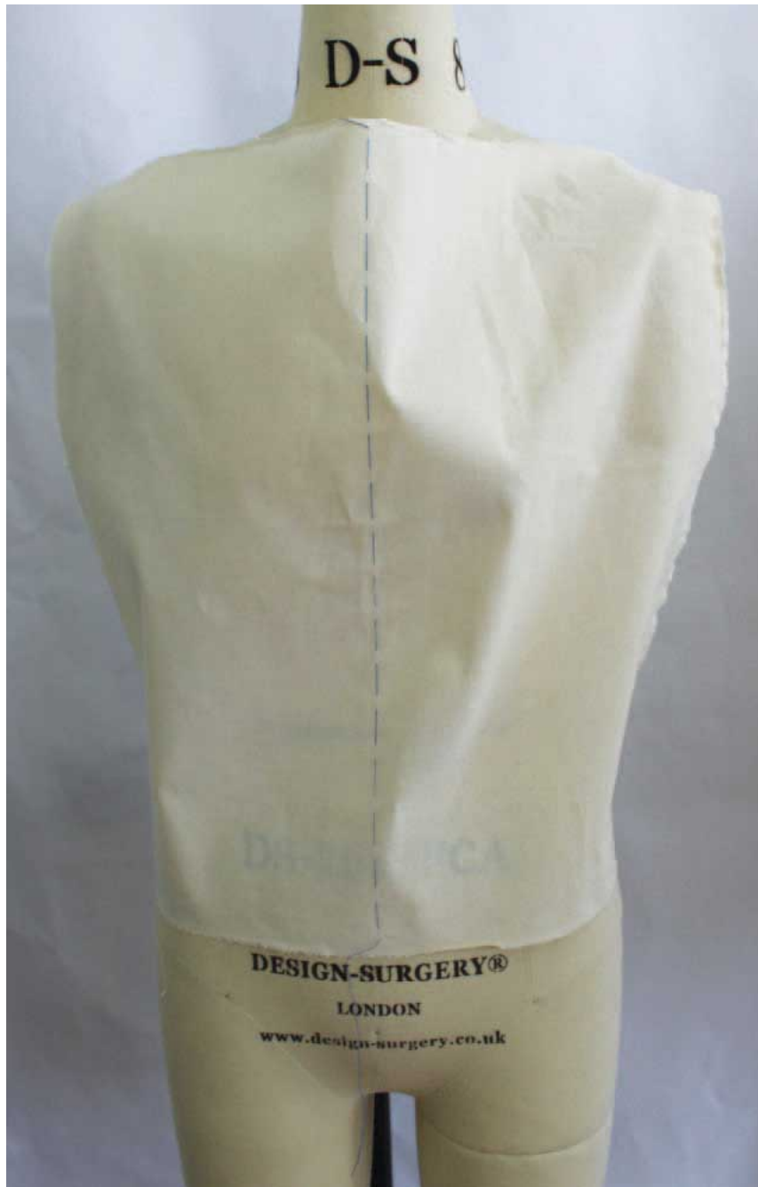
Fig. 1.17 Mediumweight calico pinned on mannequin to see the hang; grain line is marked with blue stitch line.
