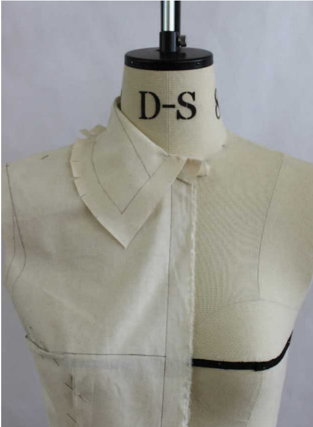
Fig. 10.35 Topcollar pinned and folded over collar stand; note topcollar finishes at CF and not at end of button wrap as per stand.
