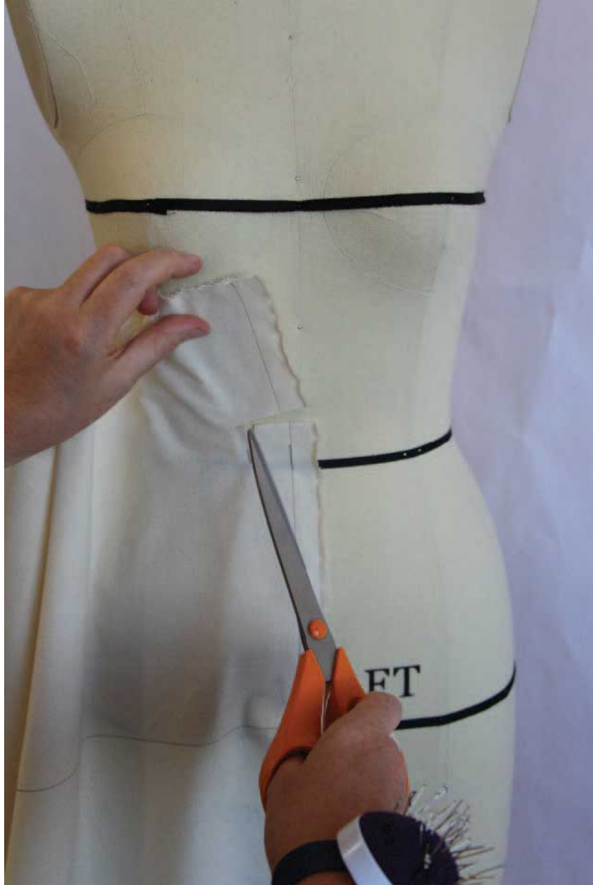
Fig. 7.29 Snipping in from CF on front quarter to start angling the volume of fabric downwards.skirt.
