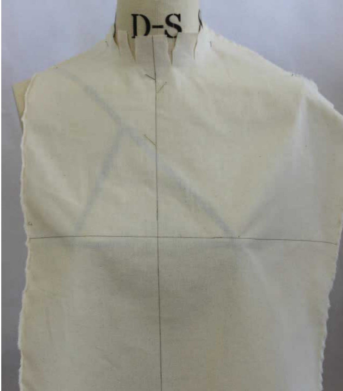
Fig. 6.45 Calico positioned for draping top panel of design that includes neckline and left armhole; neck is snipped to release tension.
