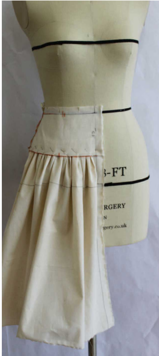
Fig. 7.49 Final drape with yoke overlaid on skirt; note series of notches added to yoke and skirt to align gathers for production pattern.
