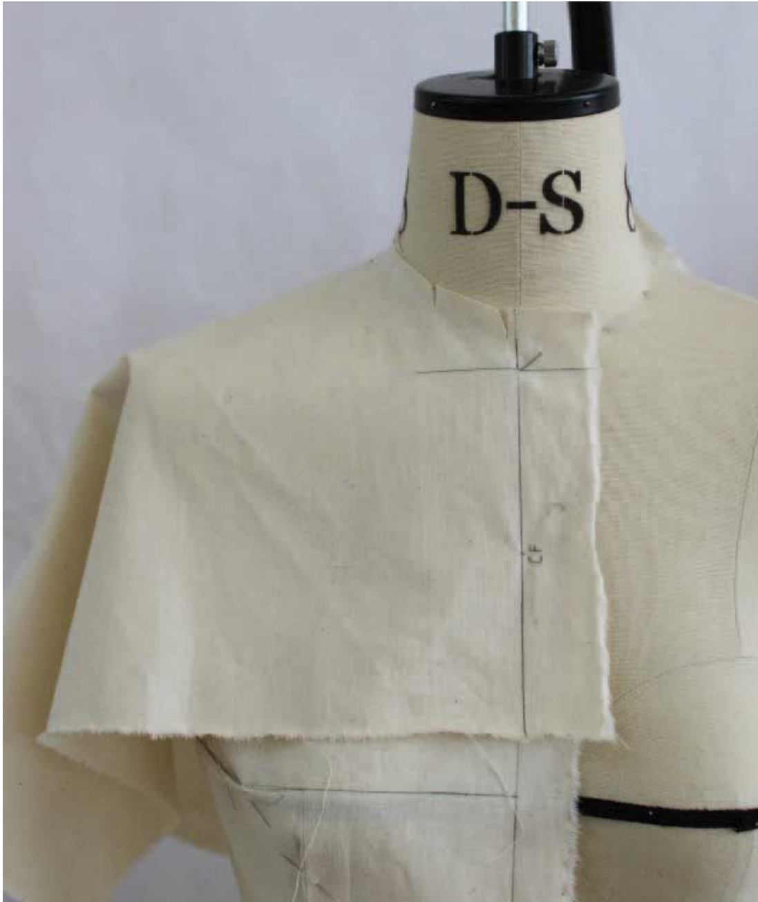
Fig. 10.6 Positioned calico lying flat to body after neck has been snipped into.
