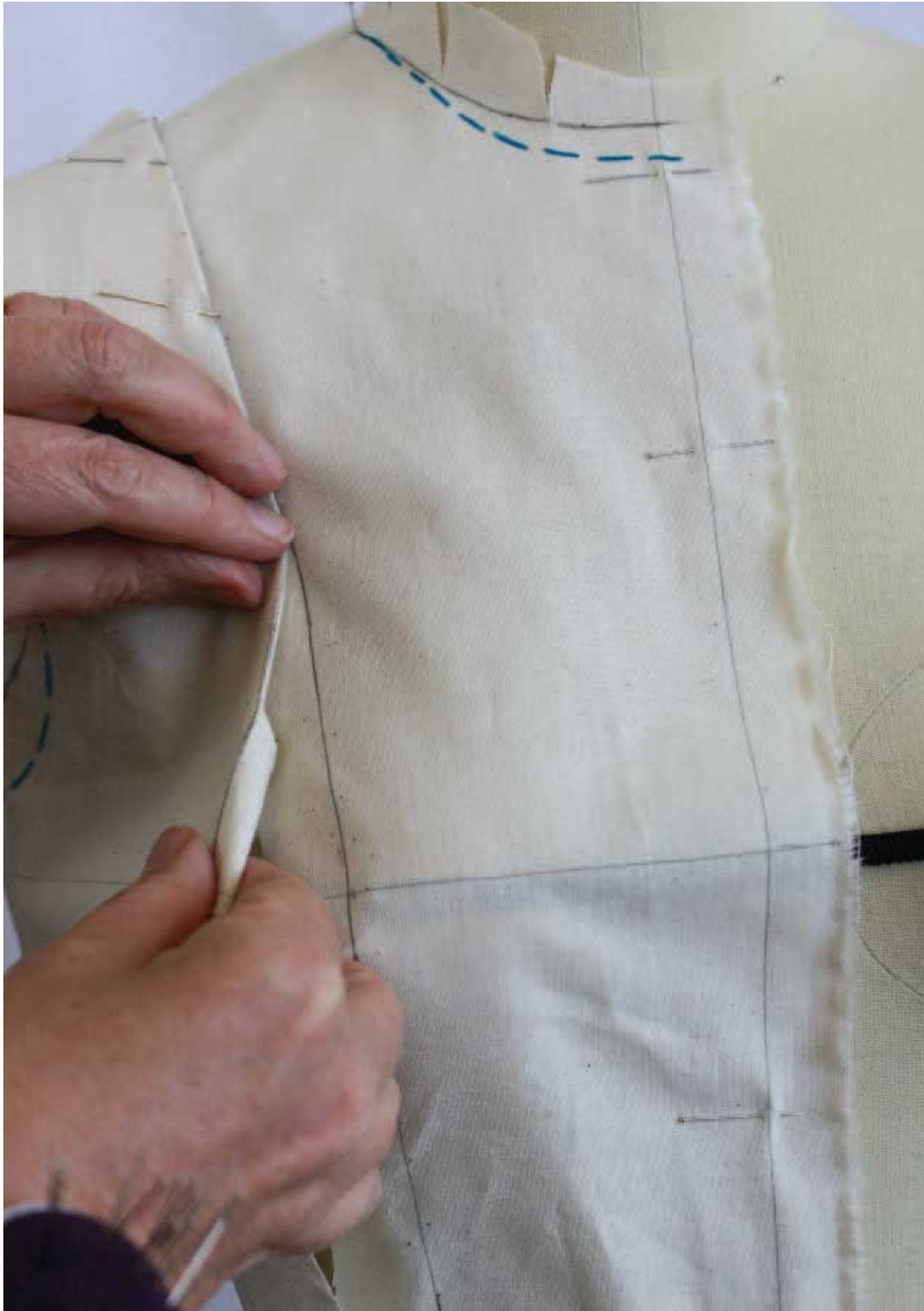
Fig. 6.36 Aligning front panels to check fit.
