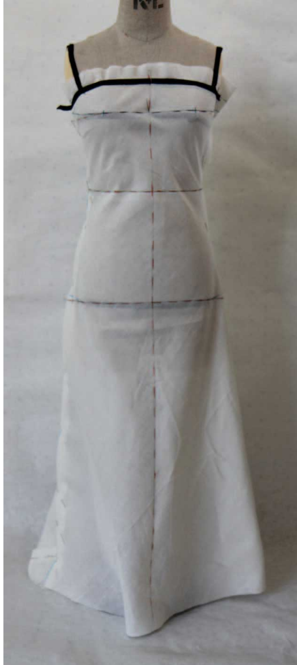
Fig. 11.12 Using twill tape to create neckline and strap position; note puckering of ease across chest.
