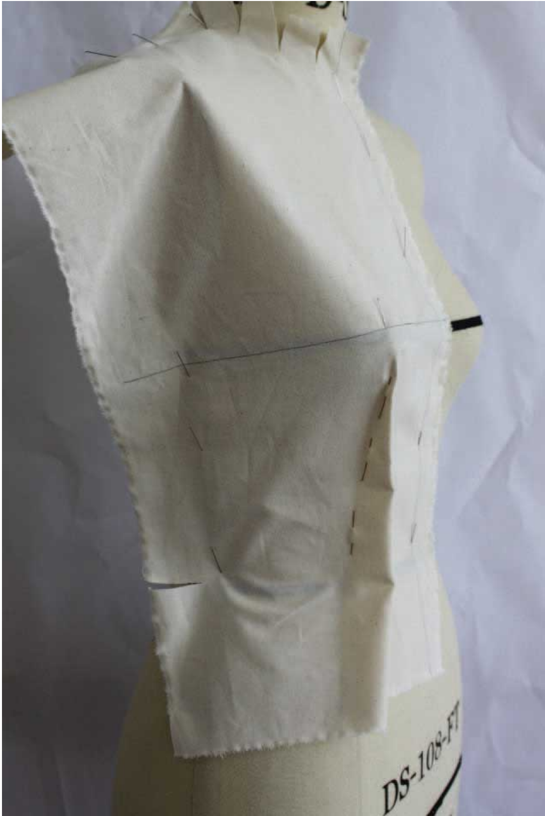
Fig. 6.4 Pinning tapered triangle or dart from BP to waist on the front of a bodice.
