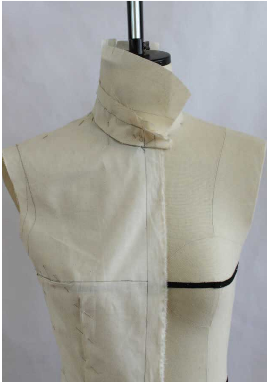
Fig. 10.34 Collar pieces pinned back together for adjustment; note extra at CF of stand for button wrap.
