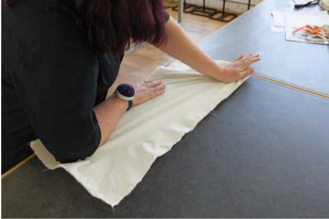
Fig. 4.9 Pushing calico grain lines back into position with the heel of the hand.
