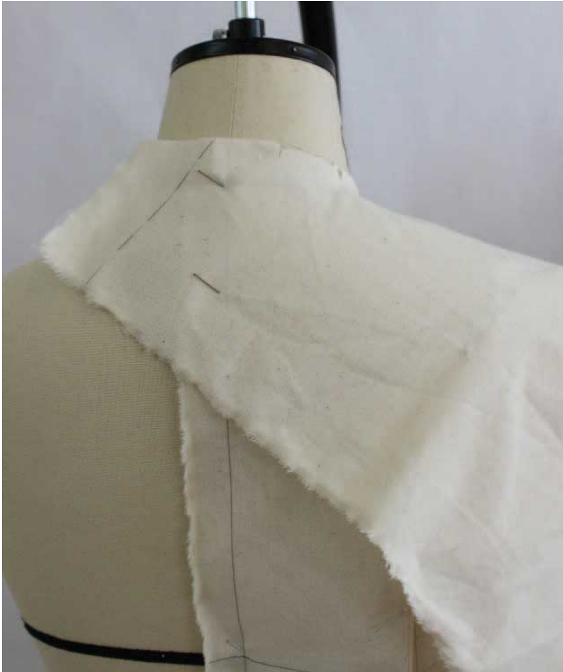
Fig. 10.5 Calico smoothed round to CB is on the bias and needs to be drawn in.
