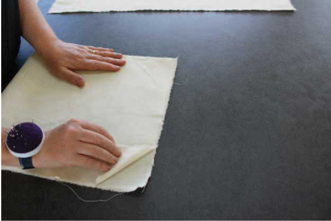
Fig. 4.11 Folding calico to check corners line up.
