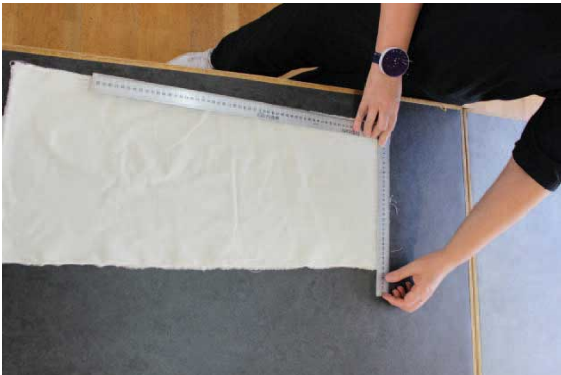
Fig. 4.10 Re-checking alignment of outside edges with L square.
