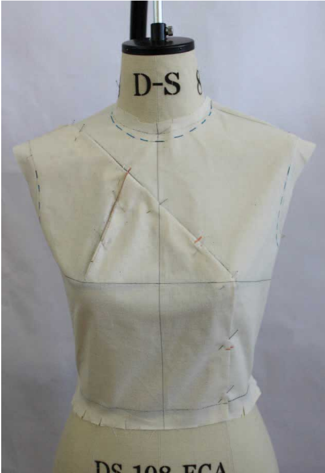
Fig. 6.52 Checking drape of asymmetric front panels.
