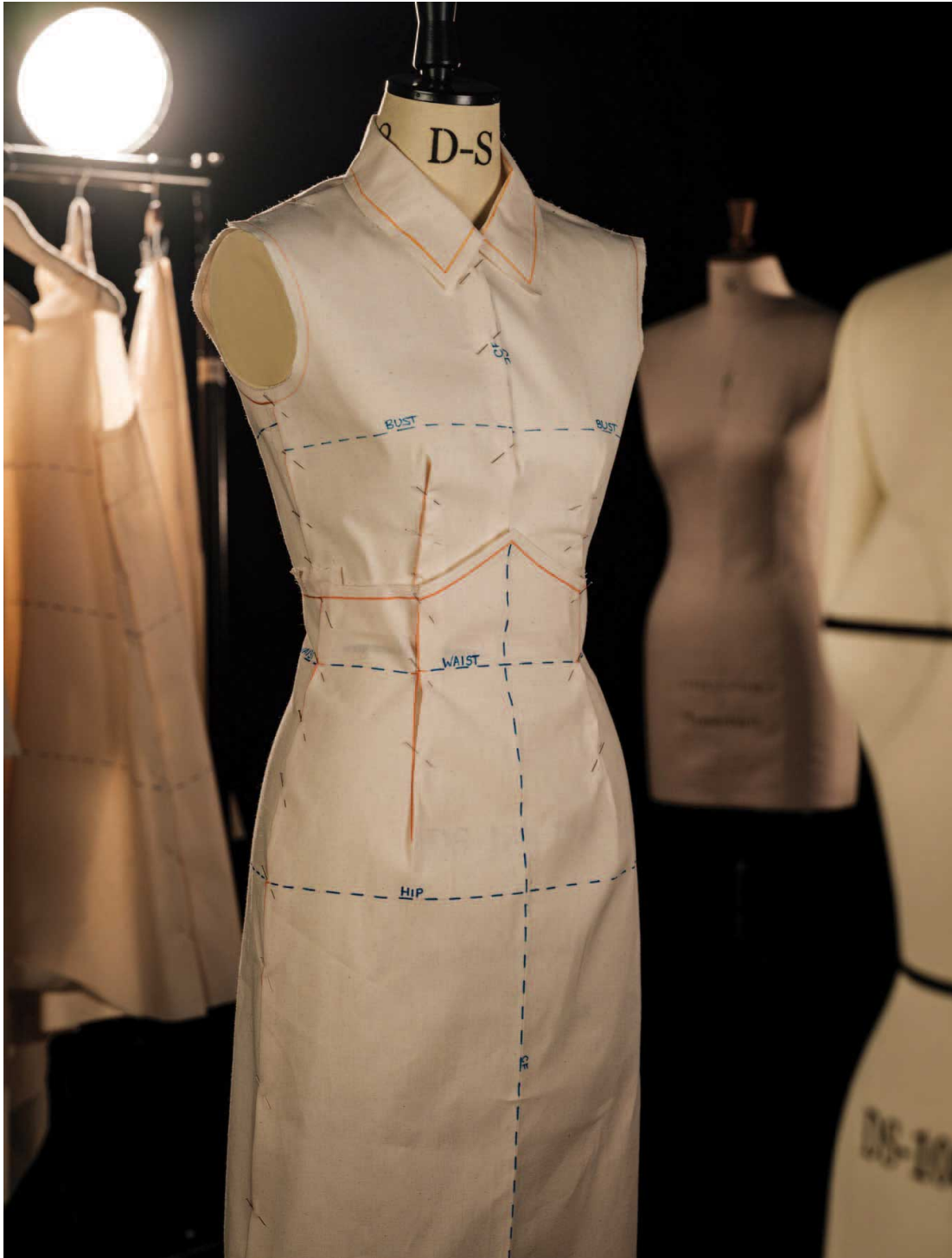
Fig. 7.8 Finished drape for high-waisted skirt with shaped waistline. (Photo: Yousef Al Nasser)
