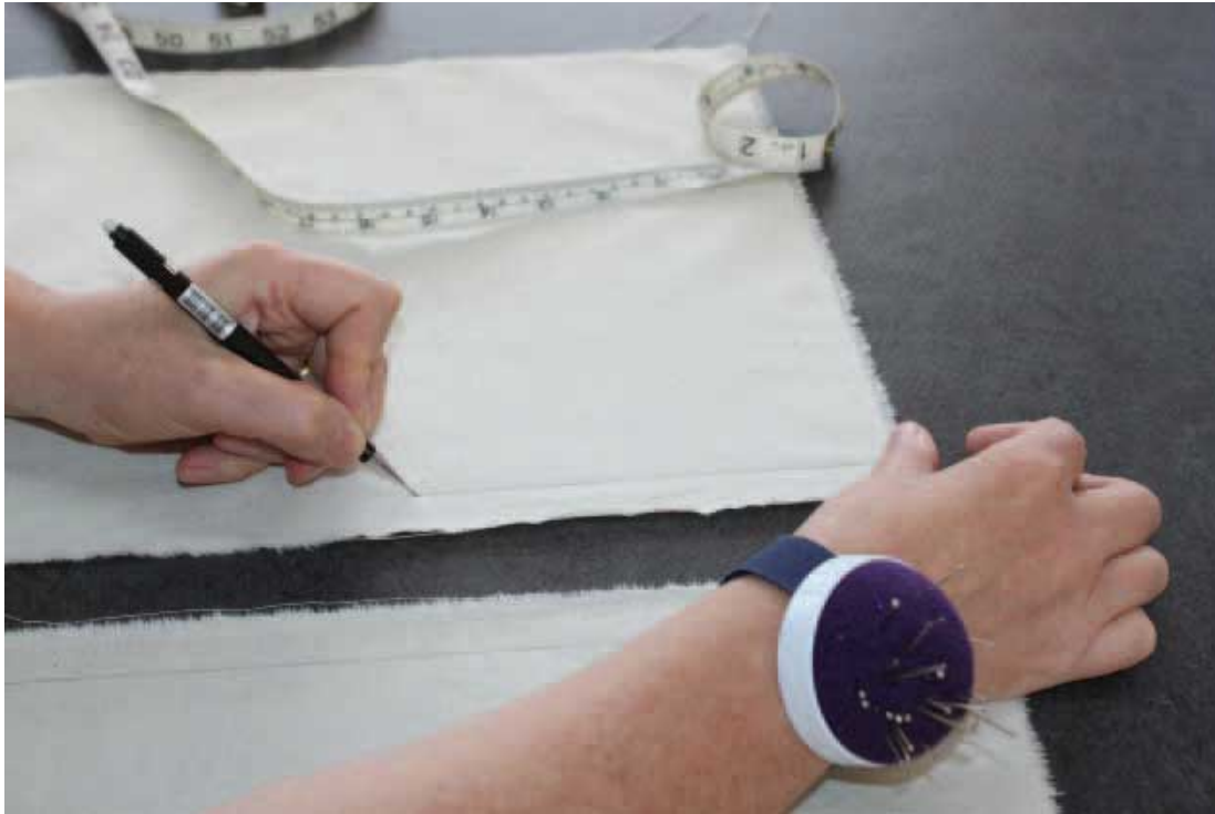
Fig. 4.14 Using drop pencil technique to draw CF and CB; note CF is on right and CB on left for a right-sided drape.
