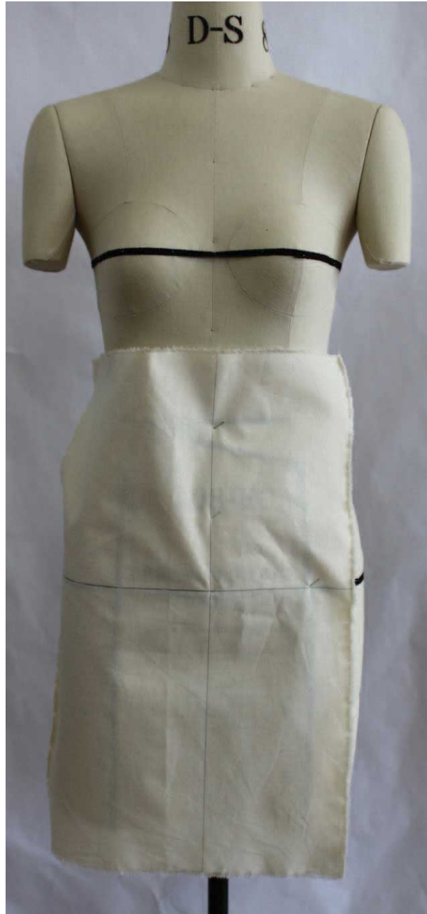
Fig. 7.17 Draping right-hand side of wrap-over skirt; calico is smoothed to SS and pinned down the style line and a dart has been created for fit.
