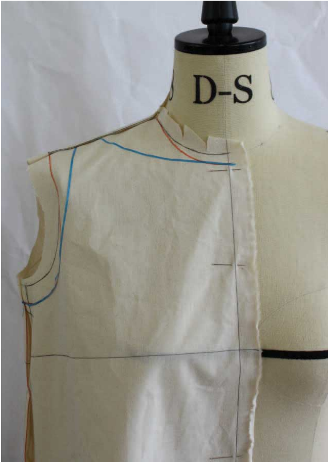
Fig. 8.39 Using adhesive tape to draw in new neckline on existing drape, front.
