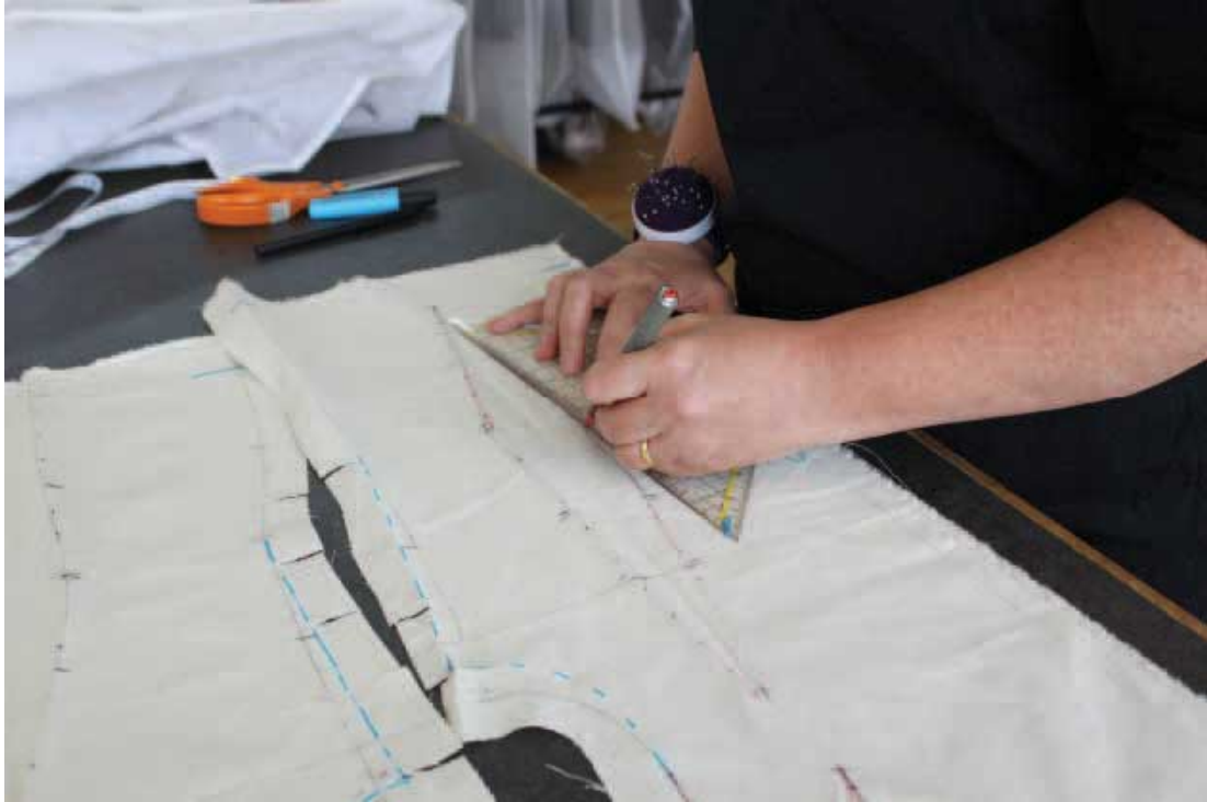
Fig. 5.5 Marking out alterations in contrasting colour.
