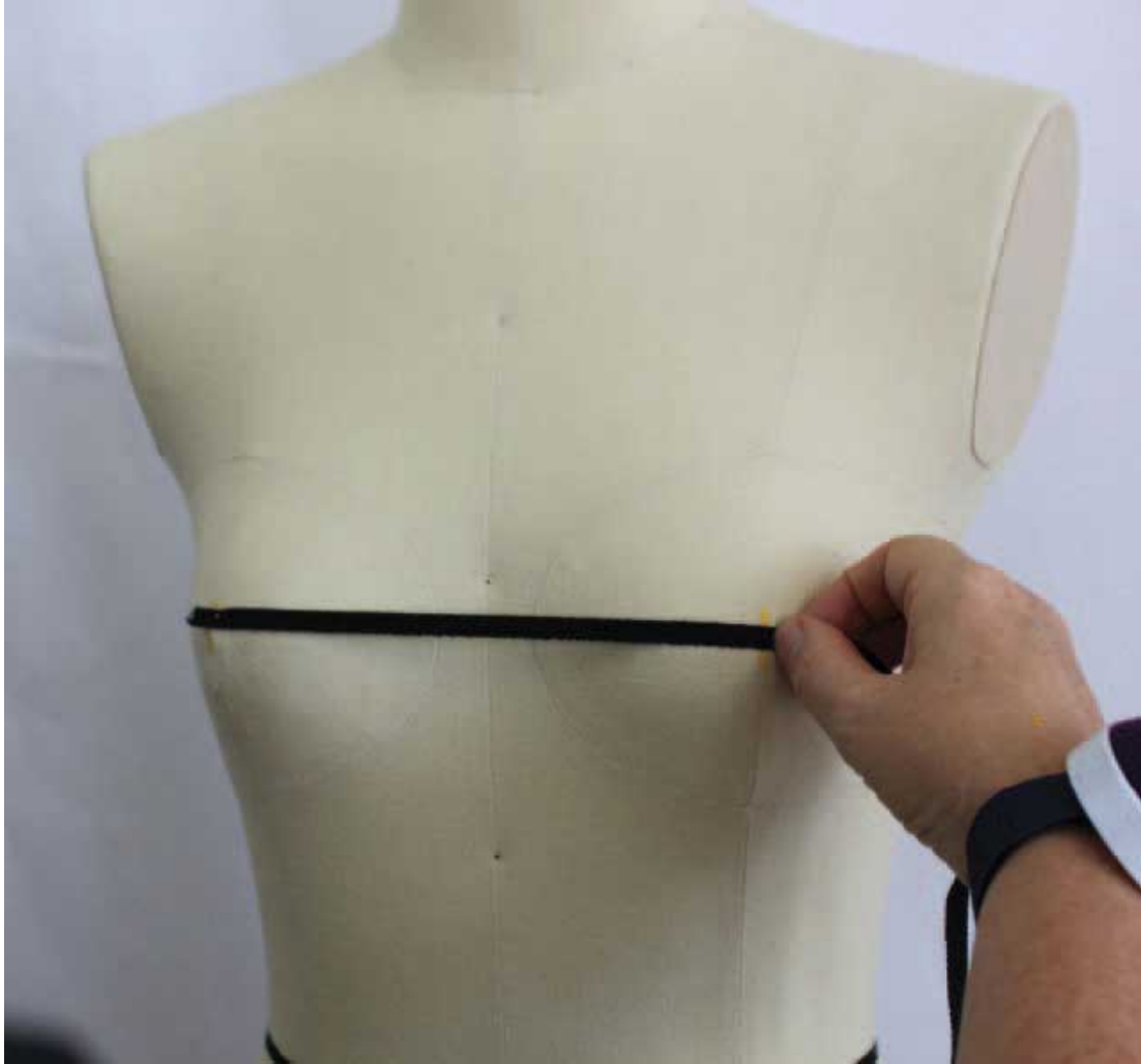
Fig. 3.7 Taping BP to BP.
