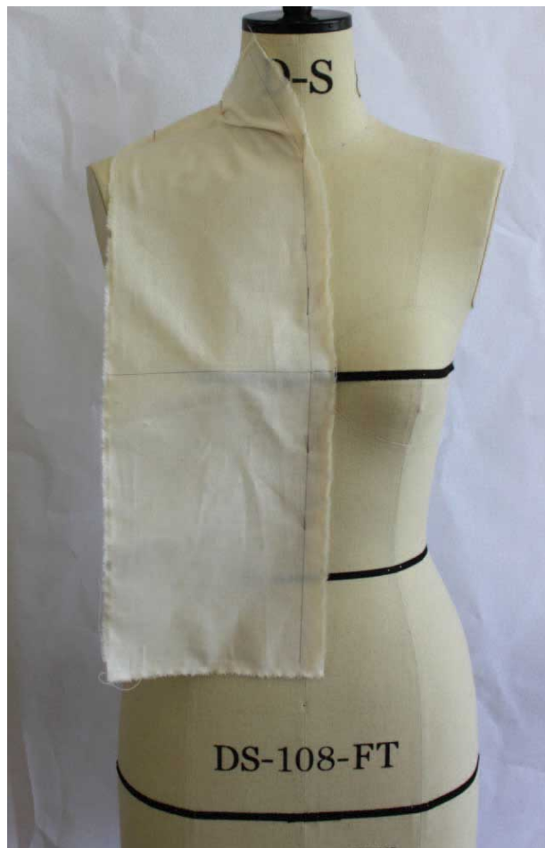
Fig. 6.32 Pinning CF panel to mannequin and aligning to where CF and bustline intersect.
