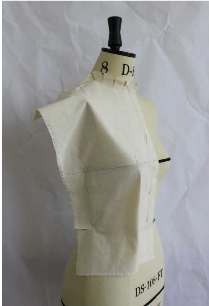
Fig. 6.14 Calico with snipped neck is smoothed along shoulder line and pinned, allowing excess volume through bust to waist to show.
