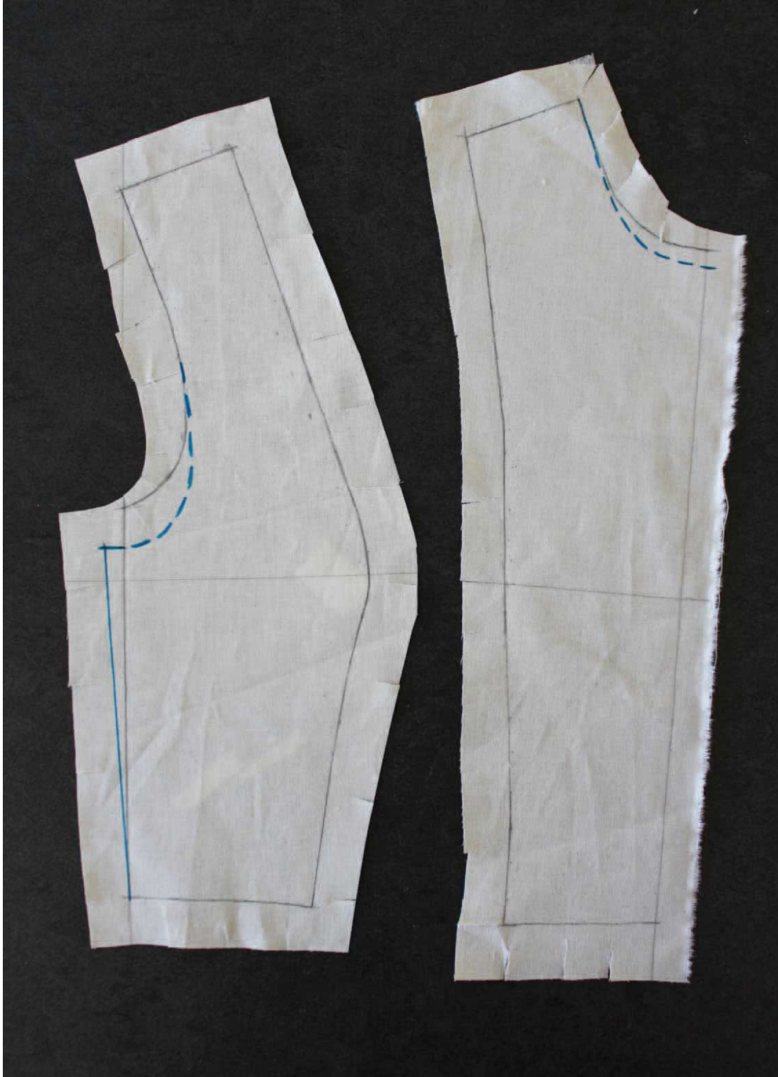
Fig. 6.33 Trued-up front and SF panels on the flat, with dropped neckline and armhole.
