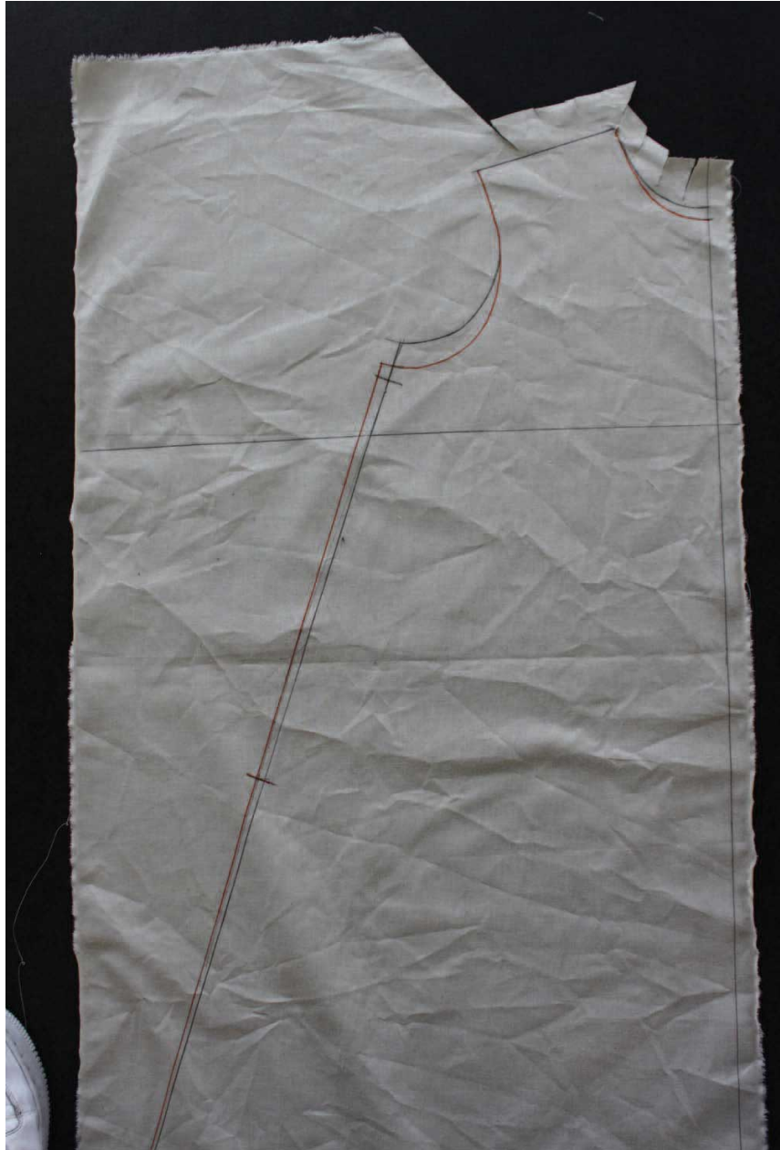
Fig. 8.36 Flared dress front on the flat; hemline is A-line shape and armhole and neck hole have been dropped.
